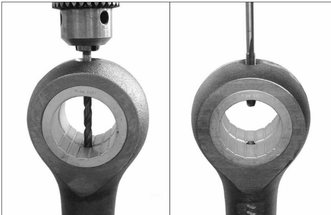
Fig. 5.1 Assembling crosshead bearing liner
